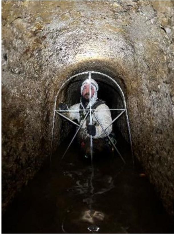
Photo 1 – Contractor performing a mandrel test on the East Fox River Interceptor.
