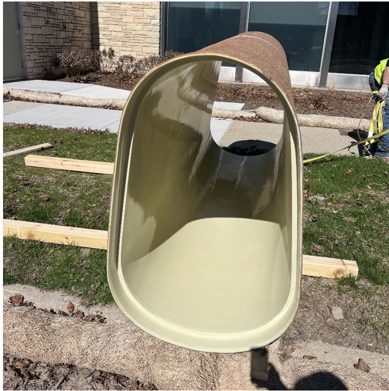
Photo 1 – 42-inch FRP pipe.
