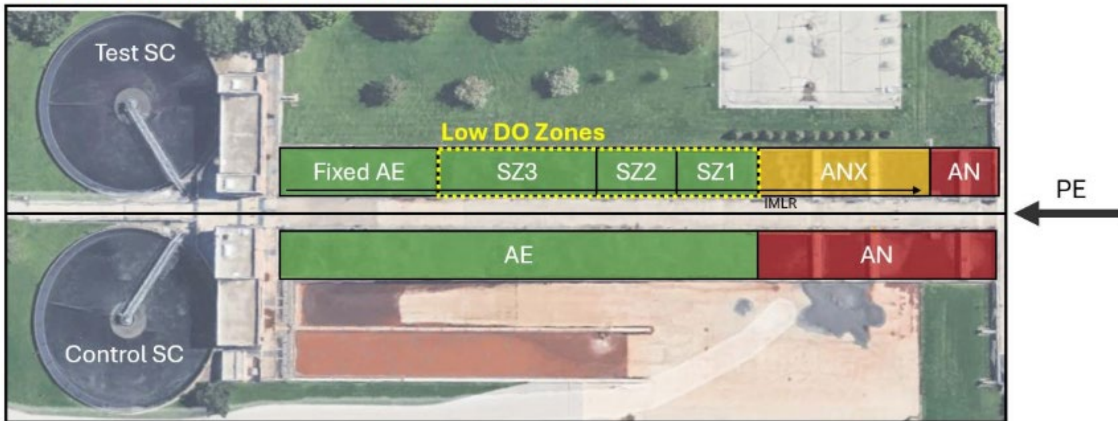
South Plant 2 (SP2) Control Train: AO Configuration
