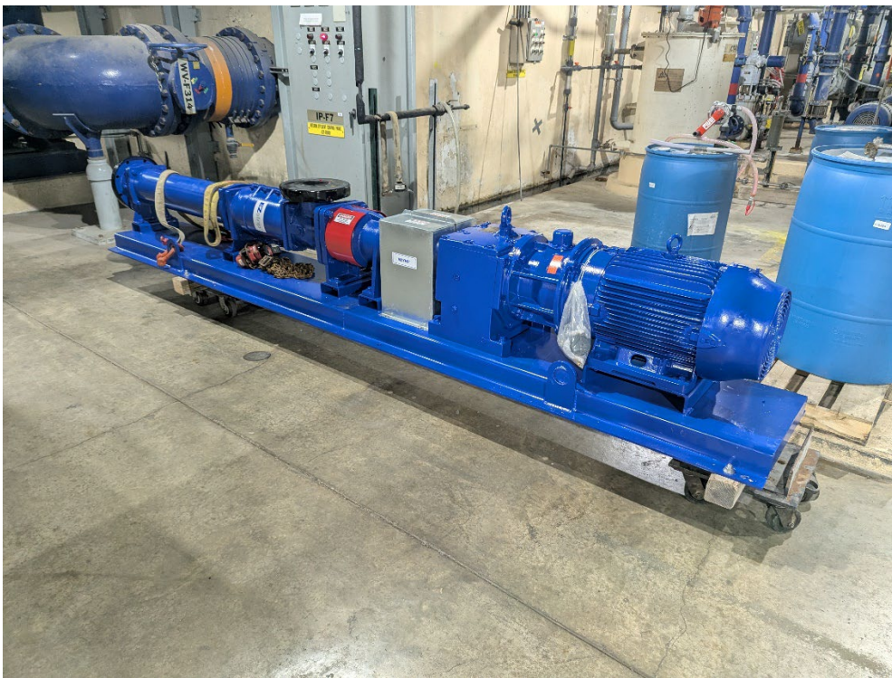
Figure 2: New Thickened Sludge Pump Pre-Installation
